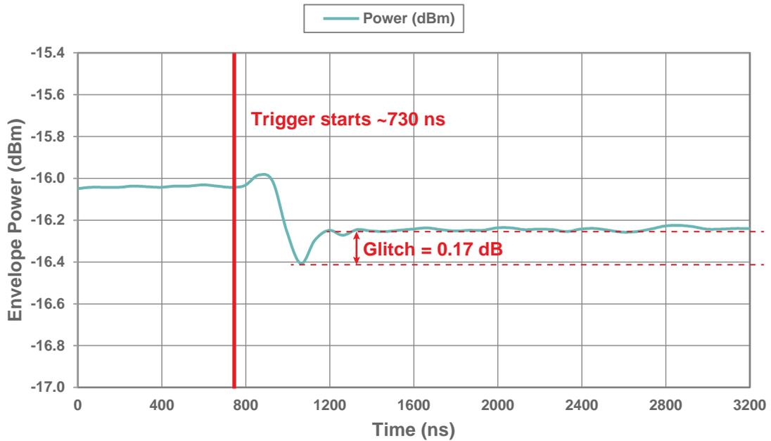
Figure 32 • Attenuation Transient (16–15.75 dB), Typical Switching Time = 275 ns
