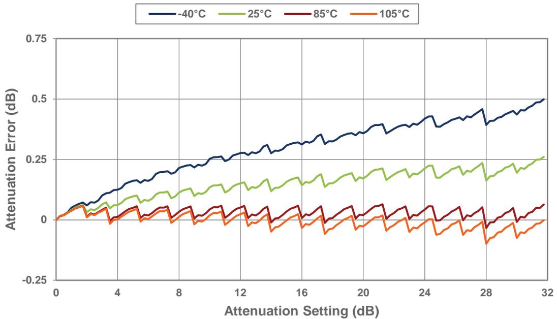
Figure 17 • Attenuation Error @ 4000 MHz vs Temperature
