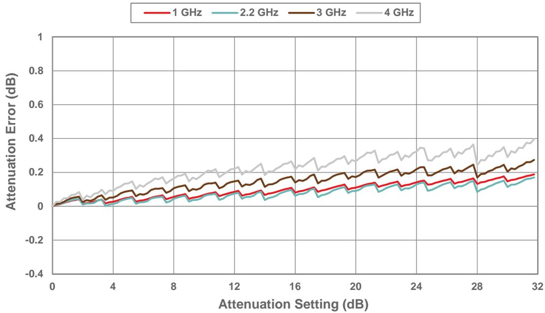
Figure 23 • 0.5 dB Step Attenuation vs Frequency<sup>(\*)</sup>
