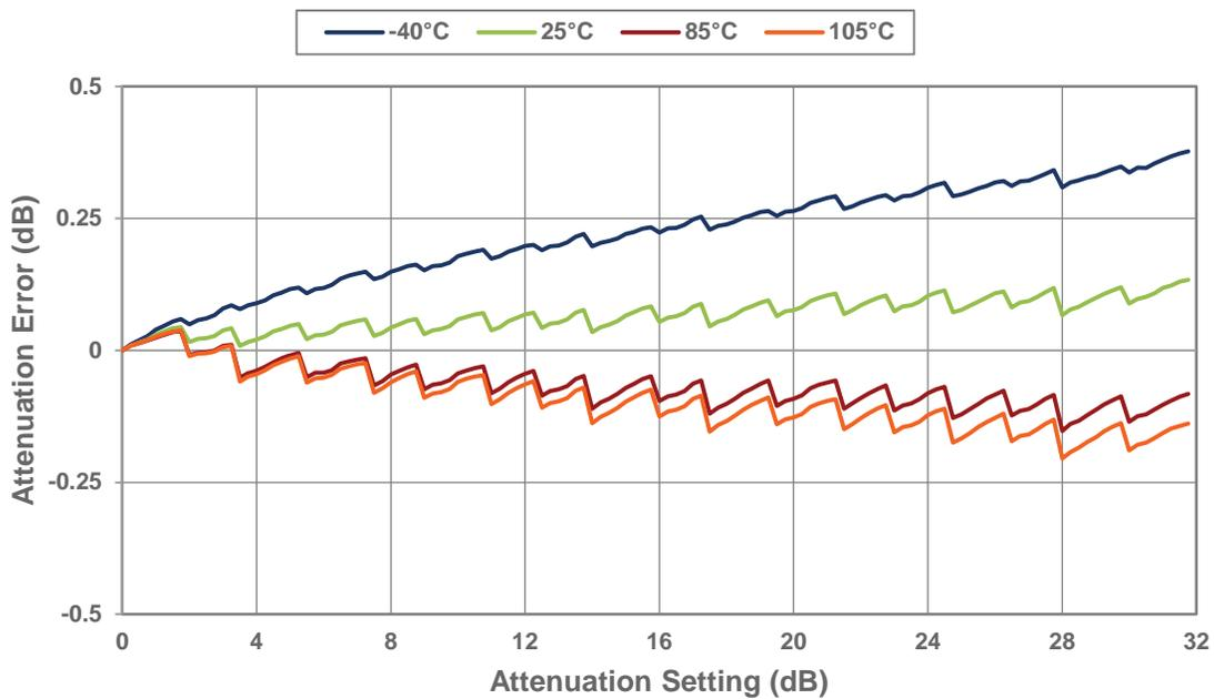
Figure 15 • Attenuation Error @ 2200 MHz vs Temperature
