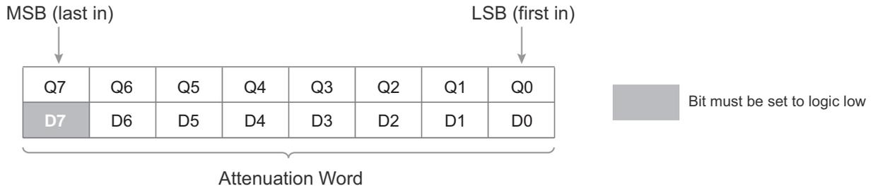
The attenuation word is derived directly from the value of the attenuation state. To find the attenuation word, multiply the value of the state by four, then convert to binary.
