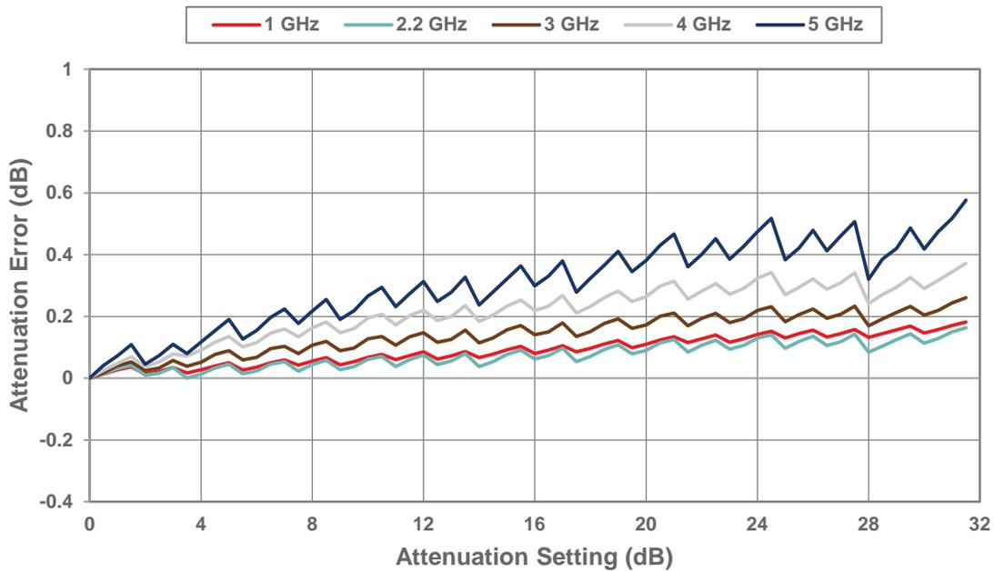
Figure 27 • 1 dB Step Attenuation vs Frequency<sup>(\*)</sup>
