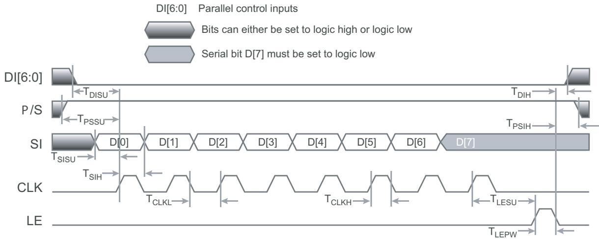
Figure 4 • Latched Parallel/Direct Parallel Timing Diagram
